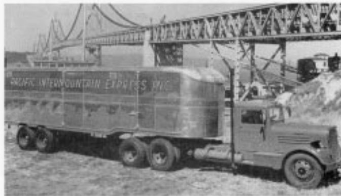
1937 P.I.E. TRACTOR AND SEMI-TRAILER Both Built By Kenworth — Chain Drive
